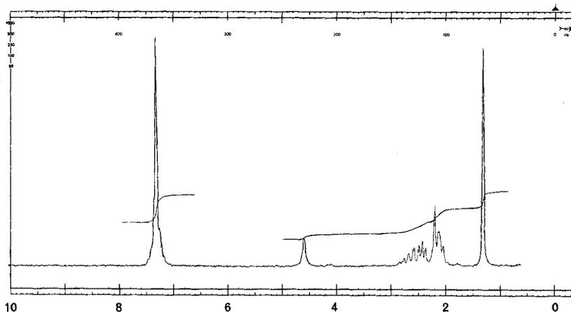
Fig. 2. NMR. ( $\text{CDCl}_3$ ) 5-Hydroxy-5-methyl-1-phenyl-2-pyrrolidon (IIa)
