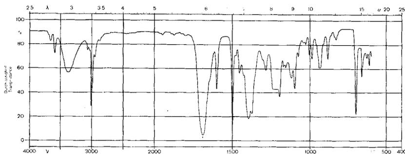
Fig. 4. IR. ( $\text{CHCl}_3$ ) 5-Hydroxy-5-methyl-1-phenyl-2-pyrrolidon (IIa)
