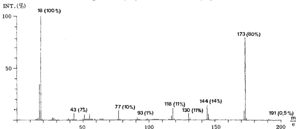
Fig. 6. MS. (45°) 5-Hydroxy-5-methyl-1-phenyl-2-pyrrolidon (II a)
